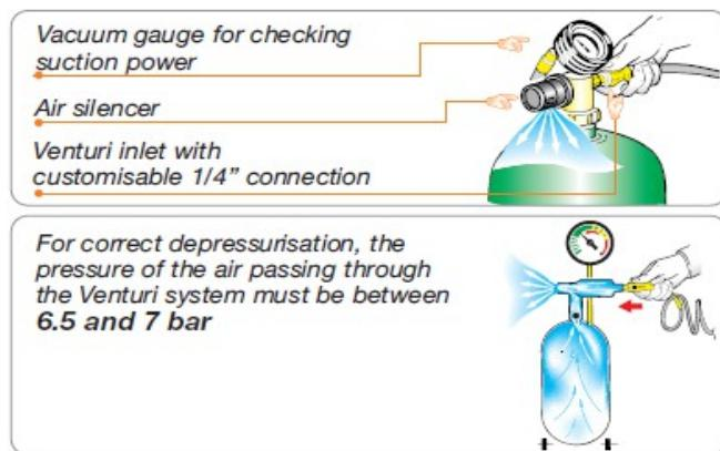
For correct depressurisation, the pressure of the air passing through the Venturi system must be between 6.5 and 7 bar
